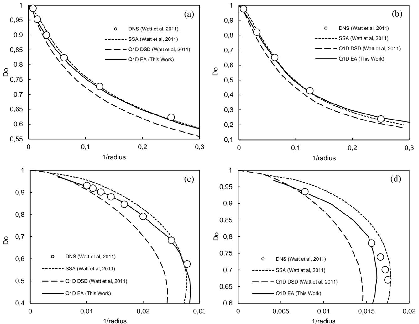
**Figure 2. Diameter effect curve for cylindrical geometry. Solid line (Q1D EA), dotted lines (SSA), dashed lines (Q1D DSD) and Circles (DNS).**
