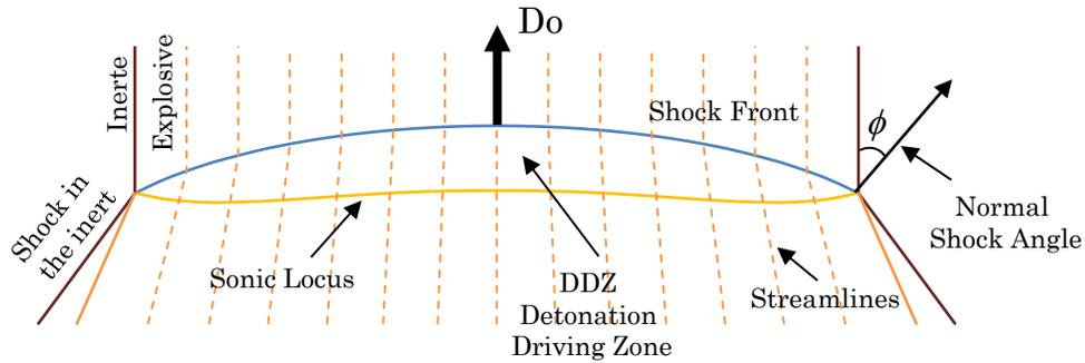
**Figure 1. Idealized scheme of two-dimensional steady non-ideal detonation. The detonation is propagating upward with a constant velocity of  $Do$ .**
