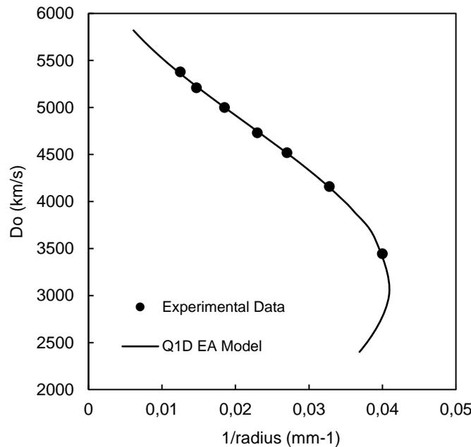
**Figure 3. Fitted diameter effect curve for experimental data for a gassed Emulsion. The CJ detonation speed is  $D_{CJ} = 6000$  m/s (19685 ft/s). Solid line (Q1D EA) and Circles (Experimental data).**
