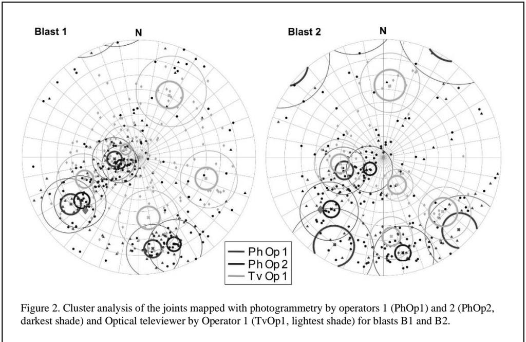
Figure 2. Cluster analysis of the joints mapped with photogrammetry by operators 1 (PhOp1) and 2 (PhOp2, darkest shade) and Optical televiewer by Operator 1 (TvOp1, lightest shade) for blasts B1 and B2.
