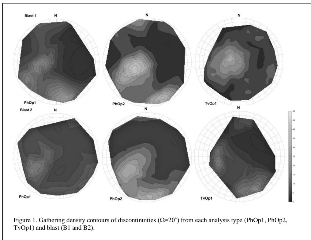
Figure 1. Gathering density contours of discontinuities ( $\Omega=20^\circ$ ) from each analysis type (PhOp1, PhOp2, TvOp1) and blast (B1 and B2).
